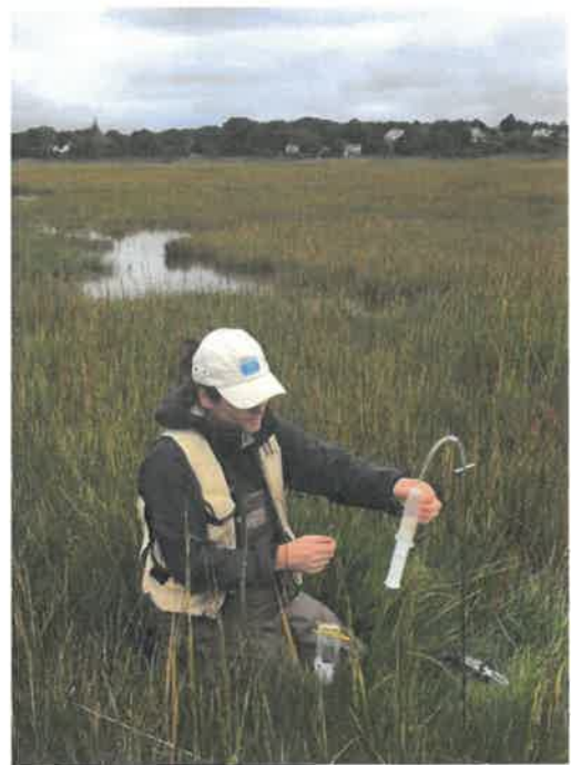
Shallow groundwater extraction from the Little River marsh in North Hampton on 9/19/18. Photo credit: FBE.
