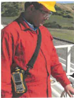
MultiRAE used for worker exposure monitoring at an oil refinery
