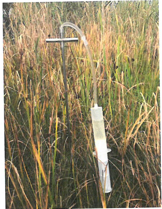
Example of a pulled groundwater sample from the marsh on 9/7/2017. Photo credit: FBE.
