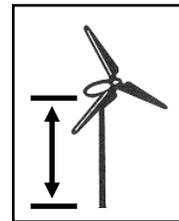
**J. Wind generator:** Blades and/or mechanical and electrical conversion components mounted on the tower associated with the conversion of the kinetic energy of wind into rotational energy used to generate electricity.
