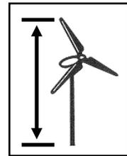
**H. Tower:** The monopole, guyed monopole or lattice structure that supports a wind generator.
